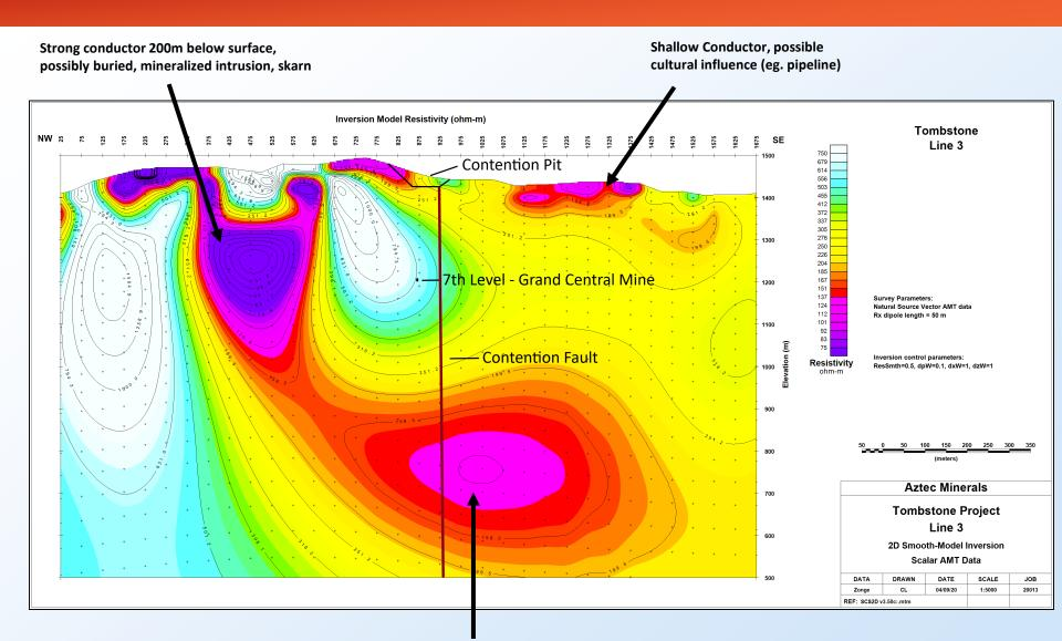
Moderate conductor 600m below surface, possible CRD massive sulfides
